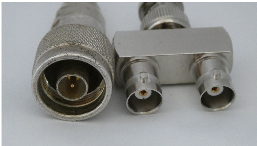
An image of an N-type plug on the left and two BNC sockets on the right
