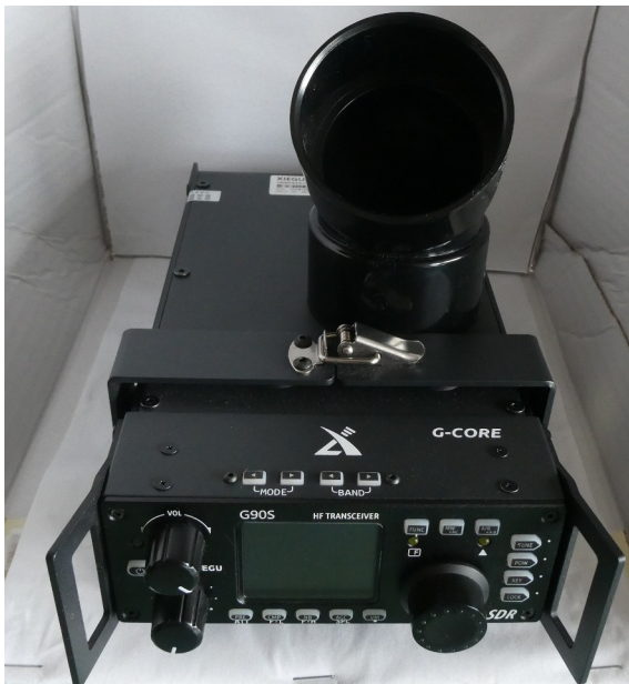
The basic plumbing part sitting over the radios loudspeaker and focusing the sound forward
