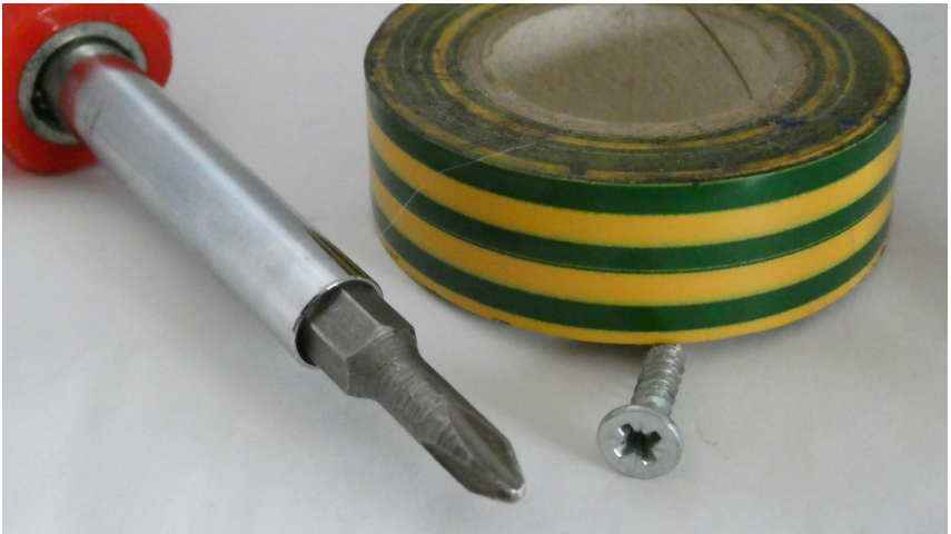
Parts needed to hold a screw onto a screwdriver
