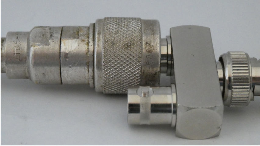
An image showing an N-type plug connected to a BNC socket
